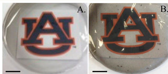
Figure 1. (A) Cast from an LSZ–SWNT supernatant added to PVA with a final film concentration of 34–4.5–61 wt % (27–4.2–69 vol %). (B) Cast from an aqueous LSZ–SWNT mixture added to PVA with a final film concentration of 4.5–9.0–45 wt % (38–8.8–53 vol %). Scalebars are 3 cm. Auburn University logo used with permission from Auburn University.
